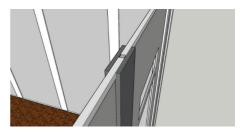
Install the clamp panel for each GRC board wall connection.
